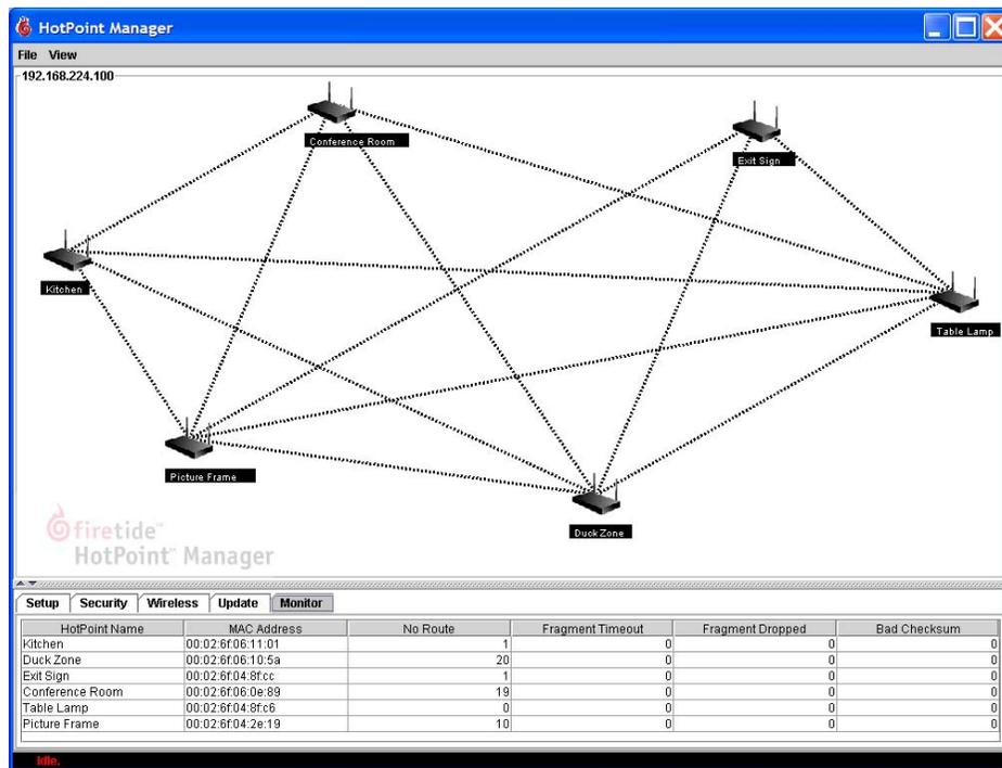
*The Hotpoint Manger Software provides a view of the mesh topology that can validate the initial design, and depicts the results of changes, moves and adds during the tweaking process.*
